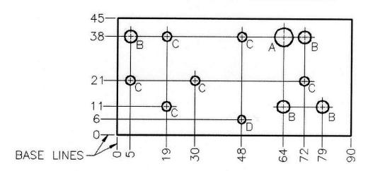
C. **Tabular Dimensioning**. Tabular dimensioning is used when a series of parts consists of the same features or geometry but vary in dimension. Letters are used in place of dimension values, and the values are then placed in a table. Most standard parts are dimensioned this way in catalogs, the machinery handbook, and in the back of most textbooks. *R1(320-321)*, *R2(471)*.
